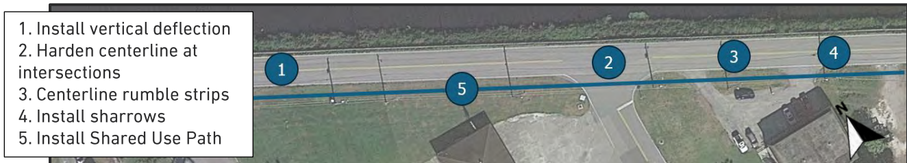
Figure 12. E Canal Street Potential Countermeasure Overview
